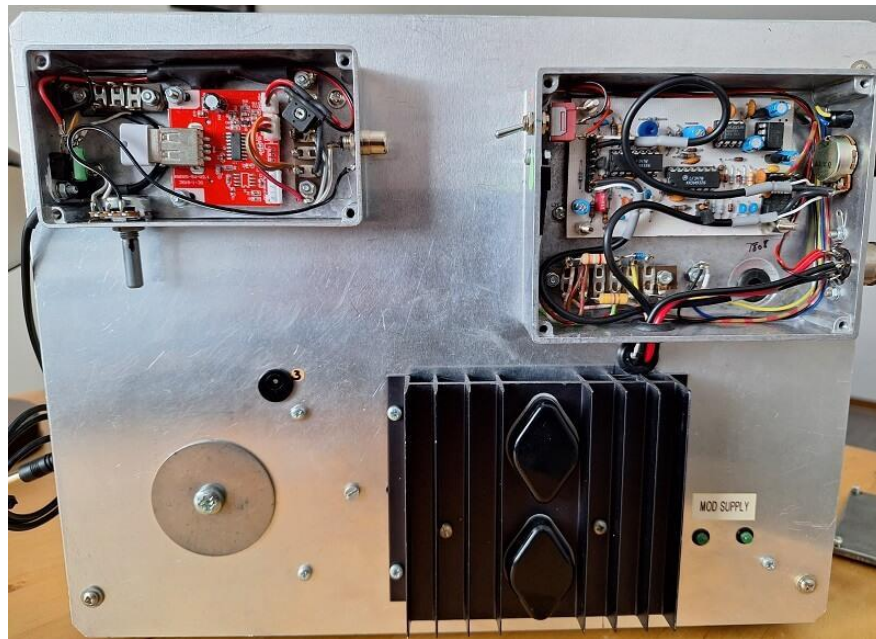
Figure 11. MP3-player (L) and the 'FAT-MAX' speech processor (R) and in their boxes
