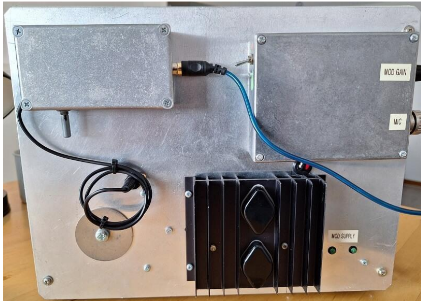
Figure 8. The heatsinks for the MOSFETS are mounted on the outside of the rear panel, together with the speech processor and MP3-player in a die-cast box
