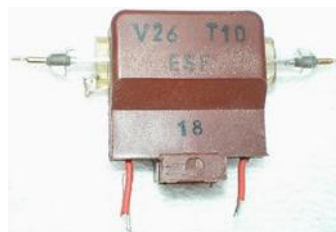
Figure 14. Reed switch used to switch the HV supply
