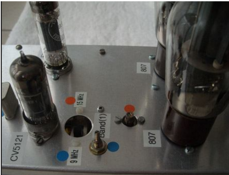
EL86, CV5121 and 2 x 807 Power Amplifier
