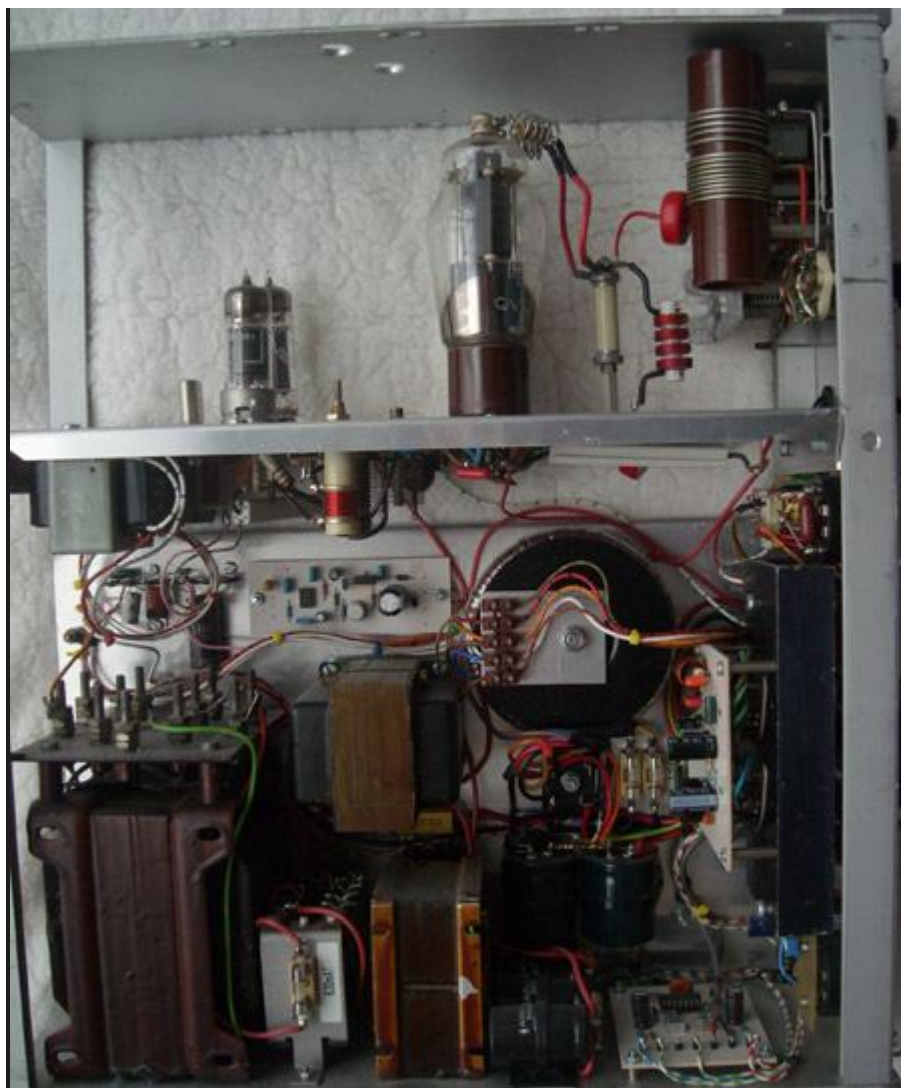
Inside the tube rig; CV5152 Crystal Oscillator, EL 86 and 2 x 807 Power
