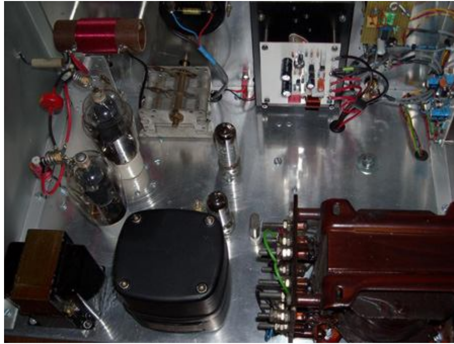
Inside the tube rig; CV5152 Crystal Oscillator, 2 x 807 Power Amplifier, PL84 clamp tube to protect the 807s in case of drive failure. Crystal on the right is the standard HC-6/U type
