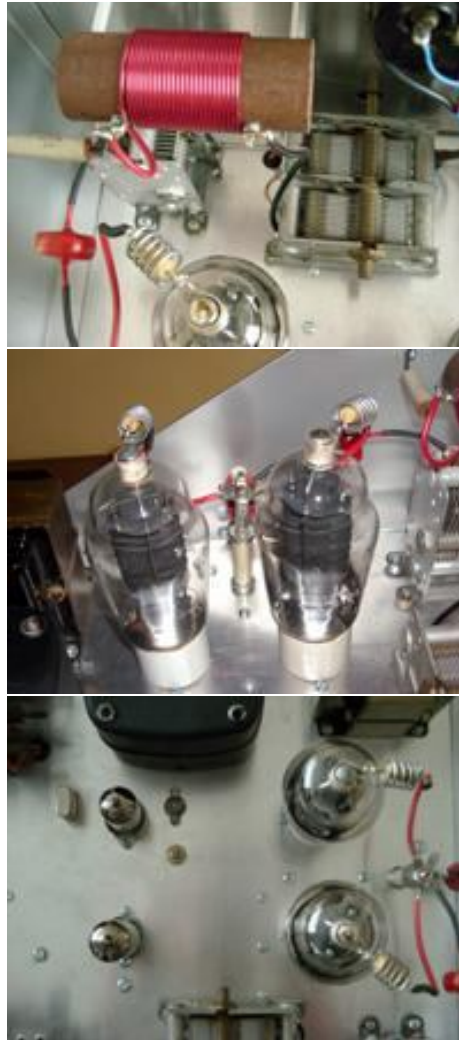
Tank circuit and 2 x 807 Power Amplifier, HT Power Supply is 525 volt / 300 mA
