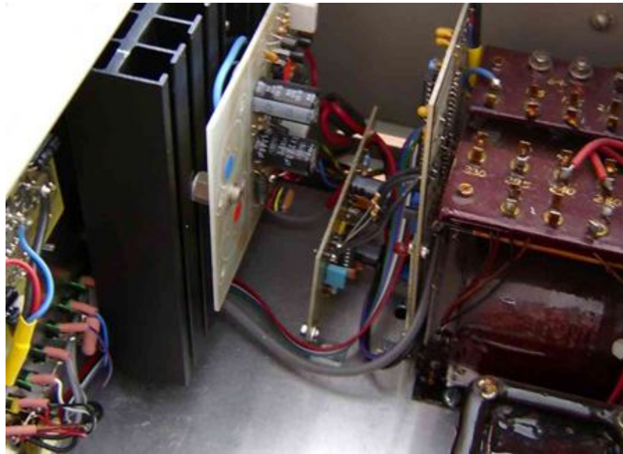
Audio section; at the left the BU2900/5, in the middle the low- and high pass audio filters and limiter
