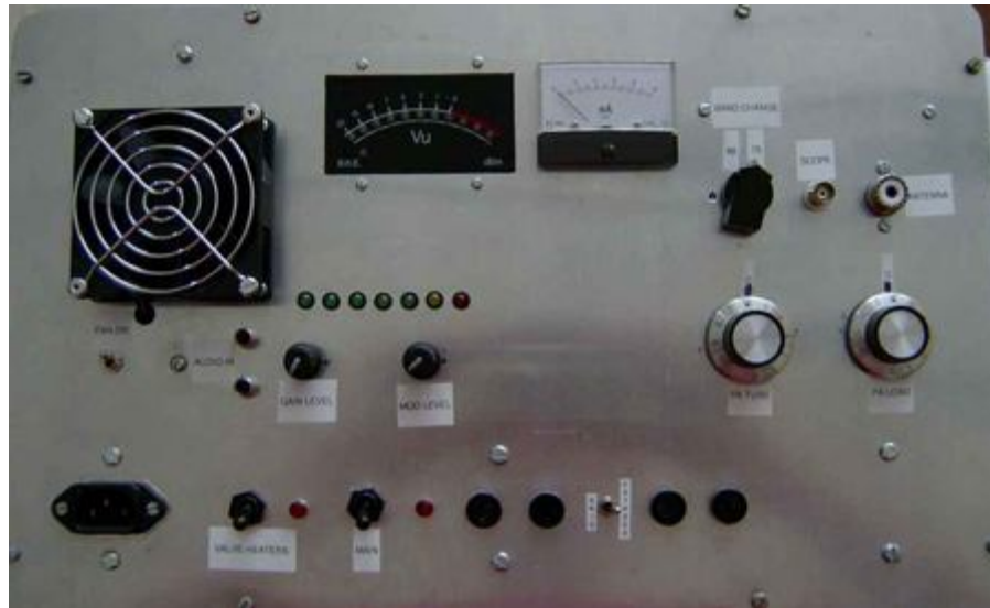
switches for gain- and mod level, grid and cathode measurement plus fan for cooling
