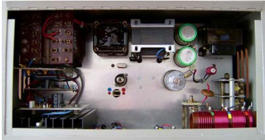
Seen from above .....below the CV4055 the frequency switch, above the crystal. To your right the 6146W and tank circuit. To your left the audio section
