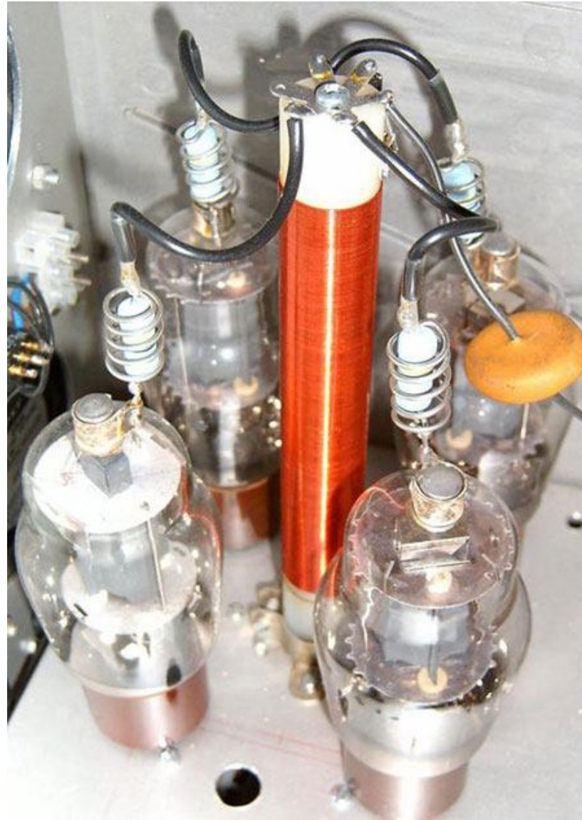
In the end-stage 4 * 807 in parallel.. nominal output power 200 Watts!
