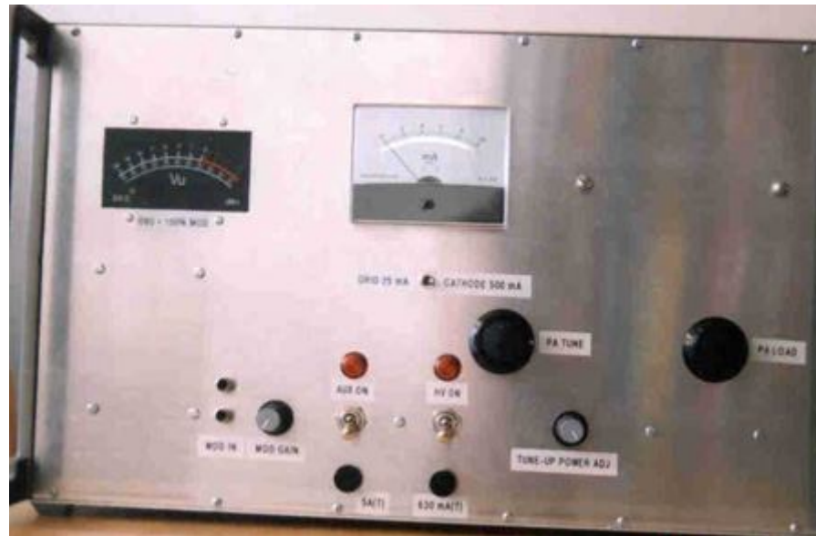
Front of the 200 Watt rig for the 76 meter band
